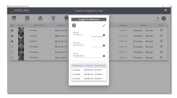
Enter the starting Static IP Address – ensure the selected addresses are not already in use by other devices on the network.
