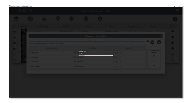
Once validated, the pop-up will close, and you will return to the CCT dashboard. The cameras to be updated will be displayed in **Cameras in progress** section of the dashboard. The new firmware will begin to be uploaded to each camera.
