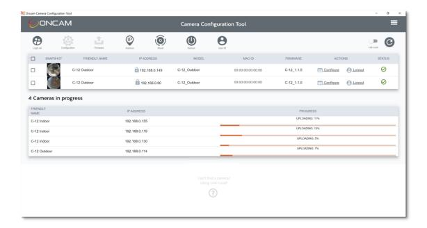
Following the upload stage, the new firmware will be installed on each camera. During each stage, progress bars will be displayed for each camera. Dependent on your network bandwidth cameras may update at different speeds.
