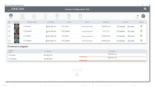
Once the reset process is complete, the cameras will be displayed in the discovered list. As the cameras have been Reset to Factory defaults, the primary administrator username and password will need to be set for the selected cameras, therefore **Set User ID** will be shown in the **ACTIONS** column for the reset cameras.
