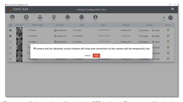
The pop-up will close, and you will return to the CCT dashboard. The cameras will be listed in the **Cameras in progress** section of the dashboard. Individual progress bars will be displayed on screen while the cameras are rebooted.
