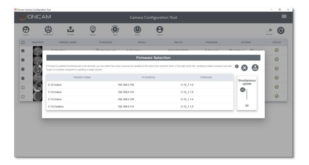
Here you can set the number of cameras to be upgraded simultaneously, by default **AII** is selected, so in this instance 4 cameras will all be upgraded at the same time. If you only wanted to upgrade 2 cameras at a time (due to network bandwidth limitations for instance), then you can use the slider on the right-hand side to set this to simultaneously update only 2 cameras at a time as shown below.
