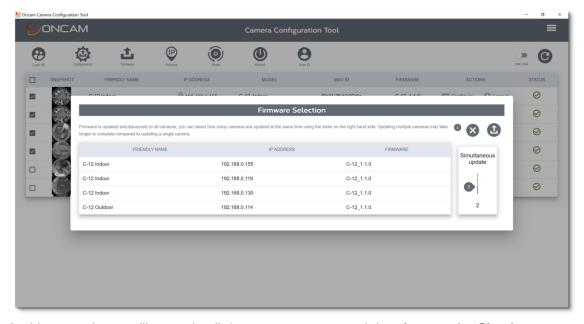
In this example we will upgrade all 4 cameras at once and therefore set the **Simultaneous Update** to **All**. Select the **Upload** button in the top right-hand corner of the pop-up, it will be highlighted in red when you hover over it.
