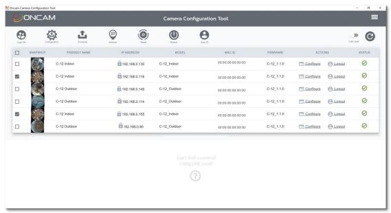
Select **Configuration** from the top menu. The following confirmation pop-up will be shown, check the selected cameras to be updated are correctly displayed then select the red button **Choose Configuration and Apply...**
