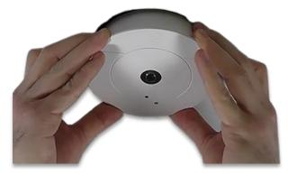
6. Carefully remove the lens protection film.
