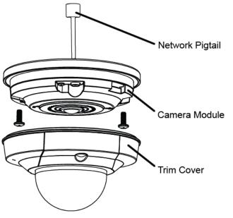
Figure 4 Outdoor Camera Exploded View
