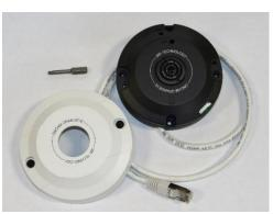
**NOTICE:** The Indoor Night camera requires an 850 nm infrared light source and passes visible, and near infrared light (850 nm).
