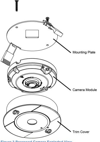
Figure 3 Recessed Camera Exploded View
