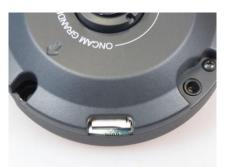
The camera uses the format EXT3, while most microSD cards use the format FAT32. Therefore, it is necessary to format the microSD card to EXT3 prior to using the first time.
