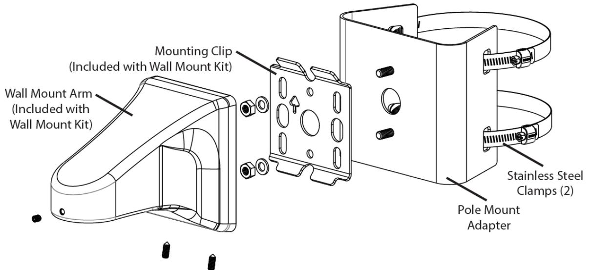
**Figure 8 Pole Mount Exploded View**
