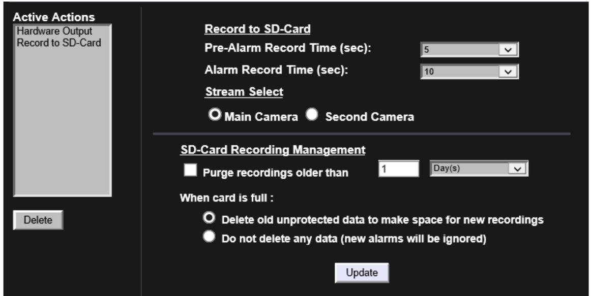
**Figure 19 Alarm Settings Actions – Record to microSD-Card**
