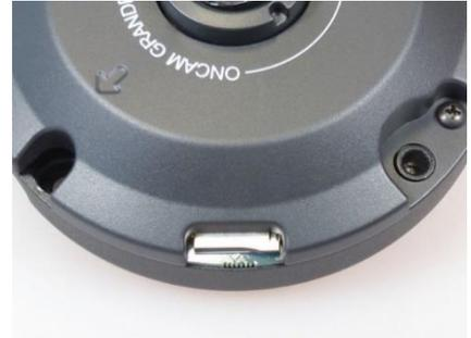
The camera uses the format EXT3, while most microSD cards use the format FAT32. Therefore, it is necessary to format the microSD card to EXT3 prior to using the first time.
