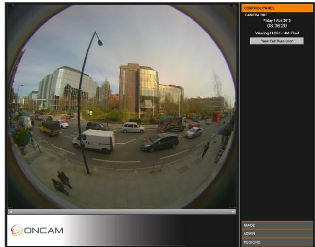
Shown in the right pane is the Control Panel that includes the camera date and time, and current image streaming.
