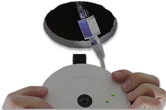
2. Connect the Ethernet coupler to the network infrastructure cable. Pass any spare cable length through the hole into the ceiling before fitting the camera.
