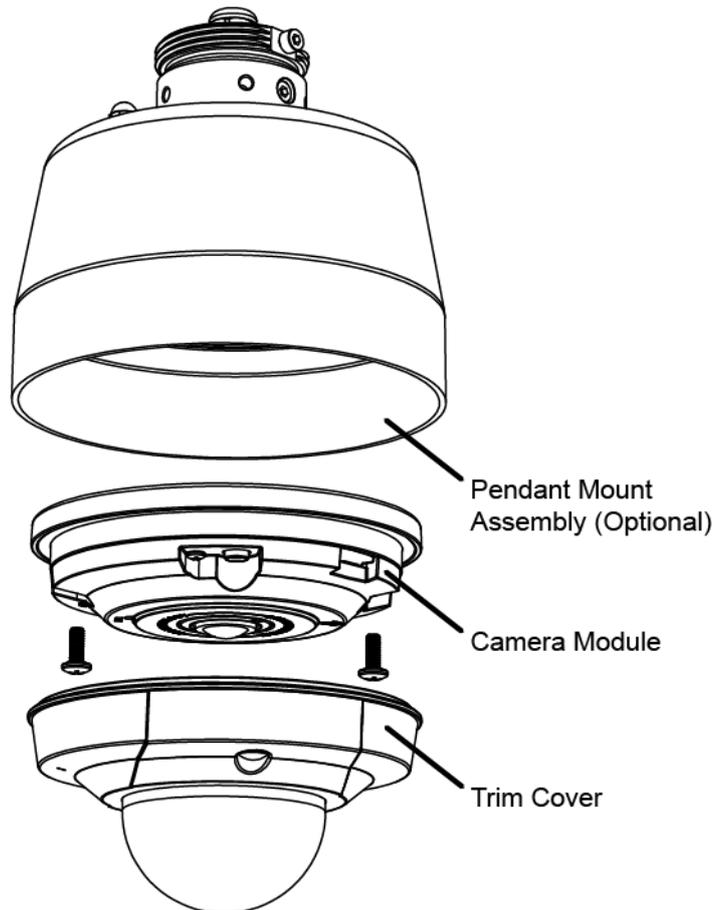
Figure 5 Outdoor Pendant Camera Kit Exploded View
