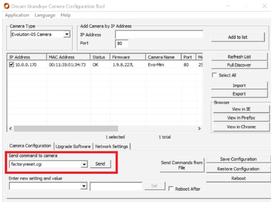
Figure 25 Camera Configuration Tool – Reset to Factory Defaults
