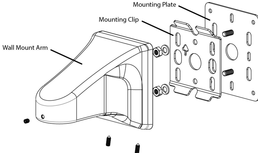
Figure 6 Wall Mount Exploded View
