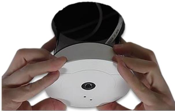
5. Release the springs and gently push the camera into position.
