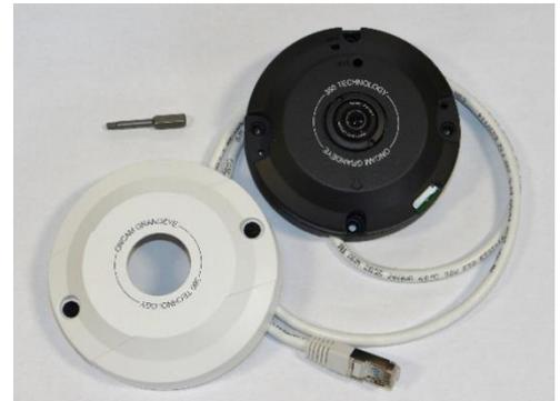
Two Torx screws attach the cover to the base.
