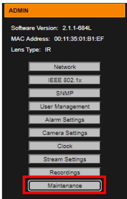
2. The Maintenance screen displays. Optionally select the Retain IP Settings checkbox.
