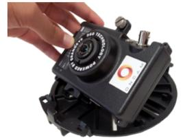
7. Fasten the Camera module with the thumb screw.
