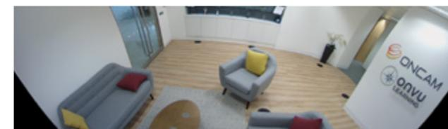
Example 6: optimized panorama from a **specialized wall mounted 180-degree** camera tilted 20-degrees down with on-board dewarping correction
